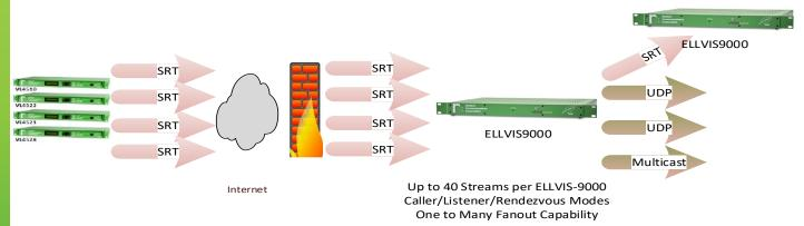
SRT optimizes streaming performance across unpredictable networks with secure streams and easy firewall traversal, bringing the best quality live video over the worst networks. It accounts for packet loss, jitter, and fluctuating bandwidth, maintaining the integrity and quality of your video.
