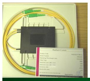
To our left, we have a unit pictured as an example. The unit is a high Isolation WDM with SCAPC connectors, installed in a ruggedized cartridge.
